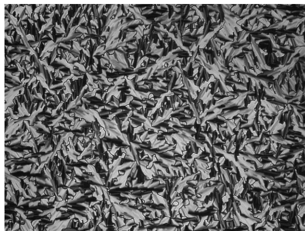
Figure 5. Optical texture of the equimolar binary mixture 1 -[ 6,4 ]/ 5 -[ 4,4 ].
