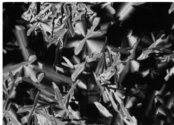
Figure 8. Optical texture of hydrogen-bonded 1/3 mixture 2 -[4,4]/5-[6,6].
